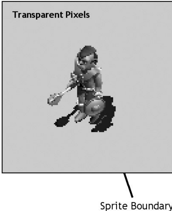
Figure 9.1 The sprite boundary is a rectangle that encloses the sprite with transparent pixels.
