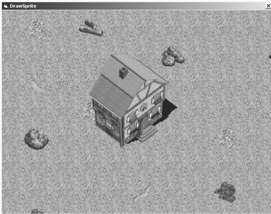
Figure 9.5 The DrawSprite program demonstrates how to draw a transparent sprite using Direct3D surfaces and textures.
